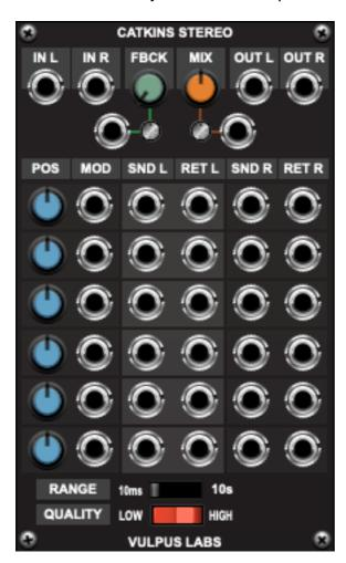
To obtain a "ping-pong" style delay with a mono input source, plug the input into **IN L**, and cross-wire the send/return loop on each delay tap so that **SND L** is returned to **RET R**, and vice versa.
