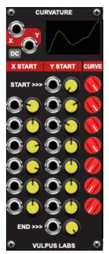
Pass an input signal into the "x" input, and take the voltage-converted signal from the "y" output.
