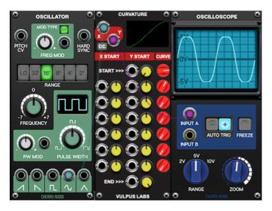
We can apply linear rectification to the signal by inverting the voltages between -5v and 0v:
