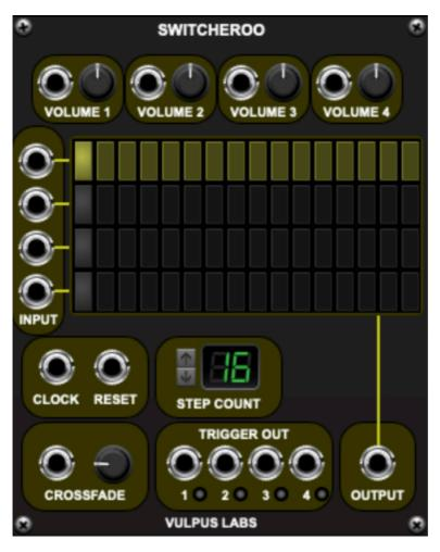
To the left of the module display are four **INPUT** jacks, to which the inputs to be switched between should be connected. Unconnected inputs will emit a silent/0v signal when switched to.
